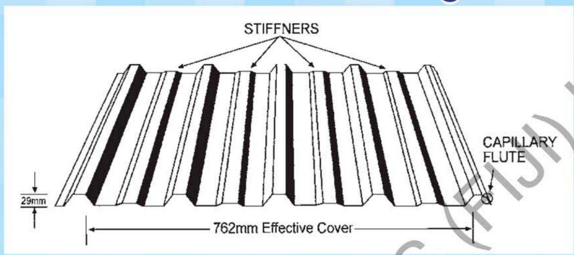
A modern, ribbed profile with stiffners in the pans to provide strength and long spanning capabilities. Capillary Flute eliminates collection of rainwater in between sheet laps preventing risk of corossion. Equally suitable for domestic, industrial and commercial applications.
